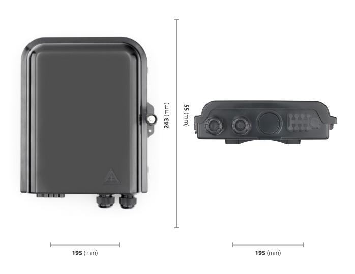
Order Code: BTNA128000B Type: Fiber NAP Boxes Application: Indoor/ Outdoor use: Splicing / Splitter IN/OUT Ports: 2:8 / 3:8 Inlet/Outlet Caliber: 12 mm / Drop-3.0 mm Max. Splice Capacity: MAX: 8 Dimensions (H\*W\*D): 243 mm \* 195 mm \* 55mm Operating Temperature: -40 °C to +65 °C
