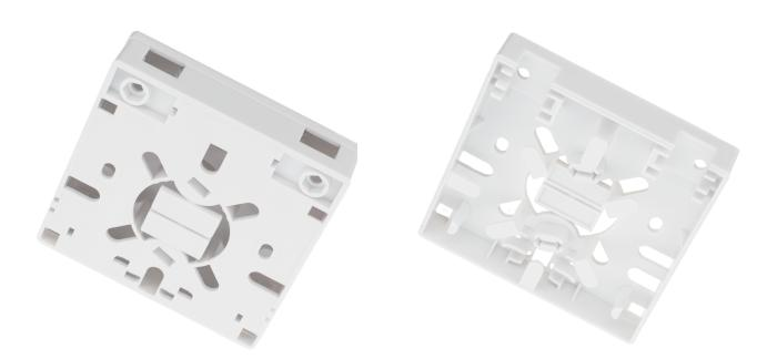
Order Code: BTOTB0511W Type: Optical Terminal Box Application: Interior of Homes and Businesses, Office Buildings and Campuses, Indoor use recommended. IN/OUT Ports: 1 /1 Inlet/Outlet Caliber: Drop - 3,0 mm Max. Splice Capacity: MAX: 06 Dimensions (H\*W\*D): 86 mm X 86 mm X 24 mm Operating Temperature: - 40 C + 65 C
