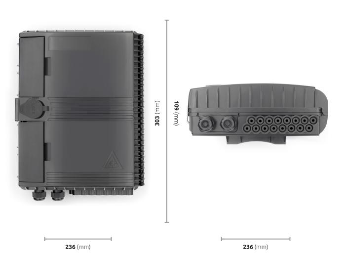
Order Code: BTFAT0811B Type: Fiber NAP Boxes Application: Indoor/ Outdoor use: Splicing / Splitter/ Cassette PLC IN/OUT Ports: 2:16 Inlet/Outlet Caliber: 16 mm / Drop-3.0 mm Max. Splice Capacity: MAX: 16 Dimensions (H\*W\*D): 303 mm \* 236 mm \* 109 mm Operating Temperature: -40 °C to +65 °C
